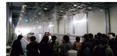
Precipitation facilities can reproduce three levels of hourly rainfall: 30 mm, 50 mm and 80 mm.
