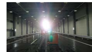
Solar irradiation testing facilities can reproduce backlight conditions including late afternoon sunlight with lights simulating the sun.
