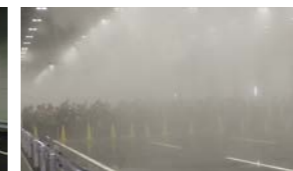
Fog generation facilities can adjust the visibility range from 15 to 80 m.
